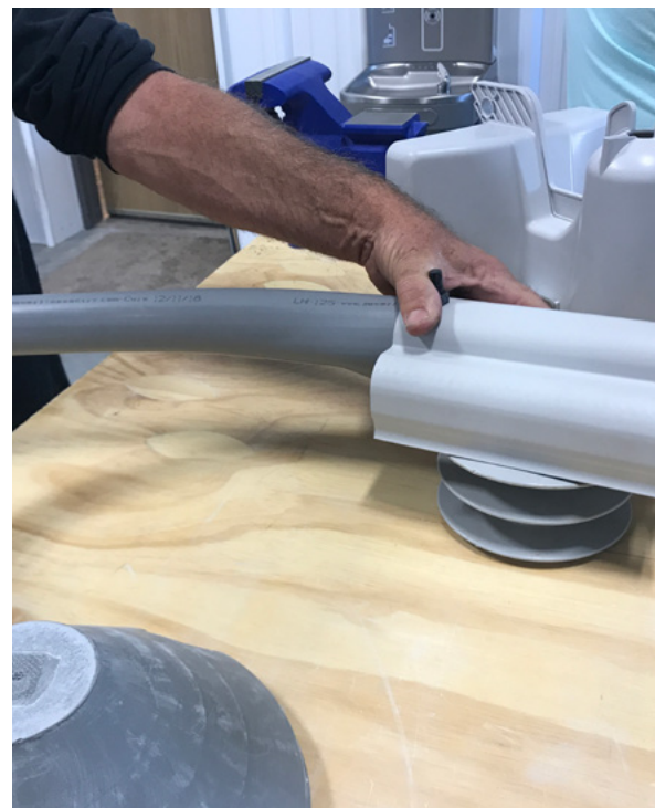
Insulation covers for distribution poles. Photo credit: Lourens Leeuwner
